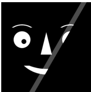
Fig. 1.2: The process of projection taking. The line integral of the brightness along the central line of a strip (shown half-illuminated) is estimated by dividing the total brightness in the strip by the width of the strip.
