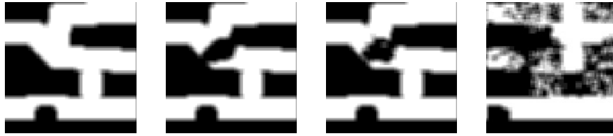
Fig. 9.3. (a) Blueprint image of a semiconductor part. (b) Test image, containing a gap in one of the wires. (c) Reconstruction of the test image from the horizontal and vertical projections, using the image from (a) as a model image. (d) Reconstruction using an inverted version of the blueprint image as a model image.
