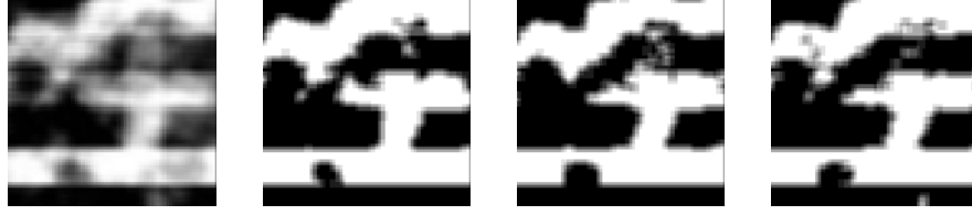
Fig. 9.4. (a) ART reconstruction of the image in Fig. 9.3(b) from six projections. (b) Rounded ART reconstruction. (c) Solution of Problem 2, using the ART reconstruction as the weight map, for lattice directions (1, 0) and (0, 1) . (d) Solution of Problem 2 using lattice directions (0, 1) and (1, 1) .
